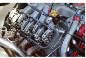
The valvetrain should be thought of as a system, explained one industry expert, "where the cam profile inputs certain dominant frequencies, and the valve springs must be able to control those frequencies without going into resonance." In turn, he continued, higher-frequency springs "allow [for] more aggressive camshafts and higher rpm limits."
