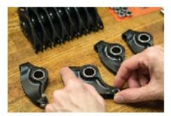
When it comes to rocker arms, design is often dictated by the material, noted one of our contacts. "We've seen an increase in demand for steel rocker arms due to their added rigidity compared to aluminum," he said, but added that it isn't always feasible to produce a steel equivalent to an aluminum-body rocker.
