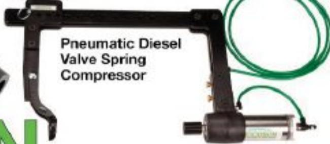
**Pneumatic Diesel Valve Spring Compressor**
