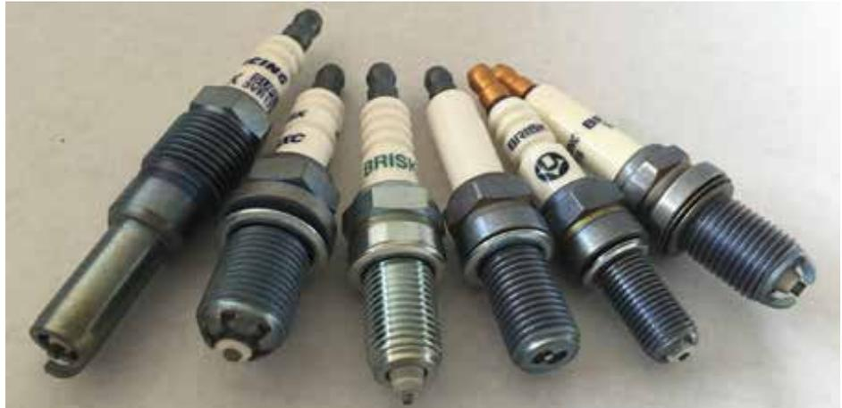
**At 5,000 rpm, each spark plug fires 2,500 times per minute (42 times/second) second, which is well within the capabilities of a stock ignition system. But in a racing application, the engine may be revving as high as 8,500 to 10,000 rpm, or even higher. At these speeds, there is less and less time for the ignition coil(s) to build up voltage between plug firings.**
