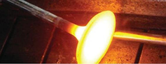
one-piece-forged, CrN-coated Tensilite titanium valves. The CrN coating offers superior resistance to impact, abrasion and corrosion; and when combined with our super-finishing process, it provides a very smooth stem with a low coefficient of friction."
