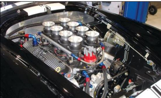
**A growing selection of available EFI products, coupled with more widespread acceptance of the technology, has created an expansive customer base that includes, among others, vintage race car owners and builders. For example, seen here is a Kinsler big block Ford Super Cobra Jet manifold with EFI installed.**
