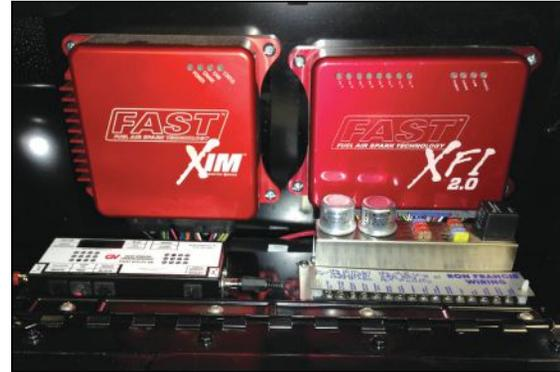
to provide a host of additional inputs and outputs directed specifically at the domestic drag racing market. Some of these features include additional injector outputs (up to 64 fuel injectors now can be run directly from the ECU/REM combination), twin solenoid (CO2) boost control, flexible torque management strategies that allow tuners to intelligently program a desired rate of acceleration (driveshaft, rpm, wheel speed, etc. can be used as
