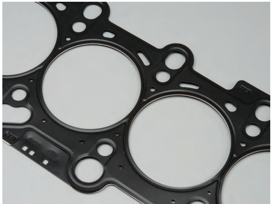
This AJUSA head gasket illustrates the "full surface" application of the polymer coating. Contrast that to the "selective silk screening" method used on the 4.6L Ford shown earlier. There's not a right or wrong method, just means to an end!
