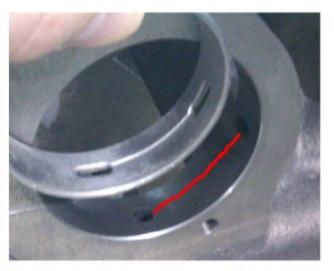
For a 60mm roller cam bearing setup with a typical distributor arrangement; do not use the standard width 20mm size roller cam bearing in the #1 cam journal location, as it interfere with the distributor shaft. Instead, use a 60mm x 12mm in the #1 journal (with Red Loctite) and the 60mm x 20mm in journals #2 - #5. Engine builds with greater than a 60mm roller cam bearing will require a distributor-less setup.
