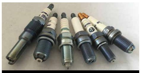
At 5,000 rpm, each spark plug fires 2,500 times per minute (42 times/second) second, which is well within the capabilities of a stock ignition system. But in a racing application, the engine may be revving as high as 8,500 to 10,000 rpm, or even higher. At these speeds, there is less and less time for the ignition coil(s) to build up voltage between plug firings.
