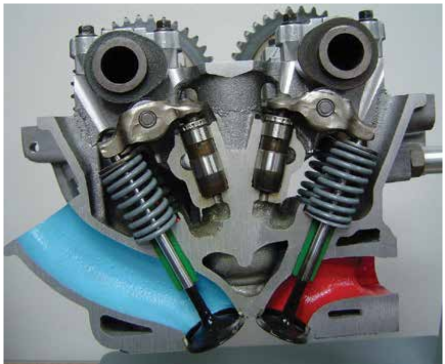
Theory is trumped by technology and reality in the valvetrain, on both the intake (left) and exhaust (right) side of the cylinder head.
