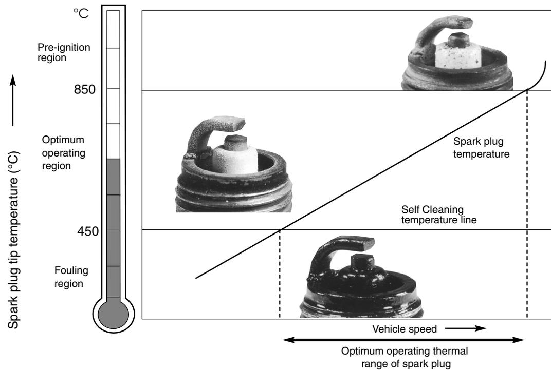
The firing end appearance also depends on the spark plug tip temperature. There are three basic diagnostic criteria for spark plugs: good, fouled and overheated. The borderline between the fouling and optimum operating regions (450°C) is called the spark plug self-cleaning temperature. The temperature at this point is where the accumulated carbon and combustion deposits are burned off.
